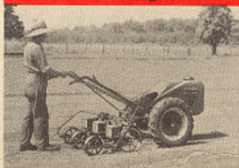
Tractor seeding three 15' rows and marking for the next gang of rows.
