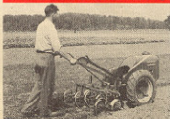
3 HP. Tractor spring tooth harrowing previously plowed stubble land.
